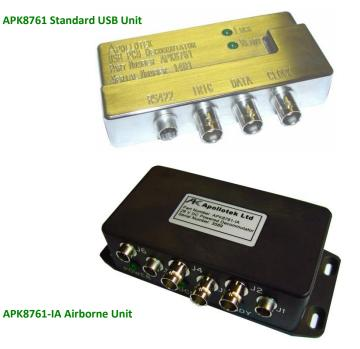
The Apollotek 8761 series of USB 2 powered miniature rugged PCM Decommutator provides Decommutation of clocked serial NRZ-L PCM data streams and provides data transfer to a host PC. Options are available to provide multiple PCM Stream outputs from a merged PCM Stream or an embedded asynchronous PCM Stream.
